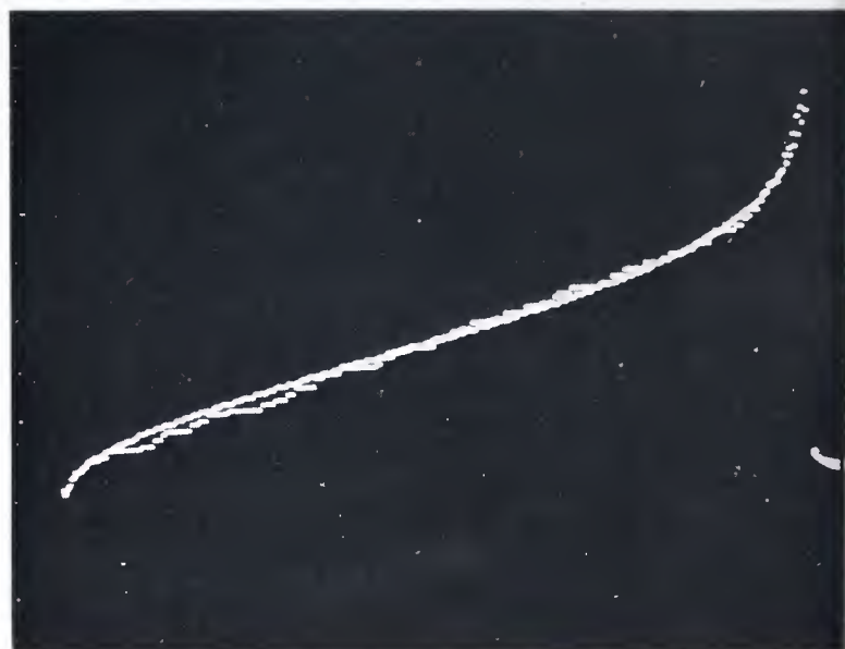
Figure 12. Local channel 1230 kHz night, Rayleigh distribution.
