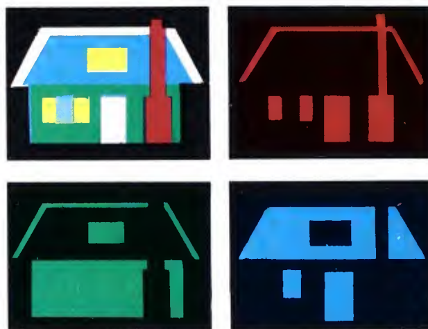
Figure 7. In the scanning process of a color image (upper left), the color camera separates the subject into three color image counterparts for transmission.
