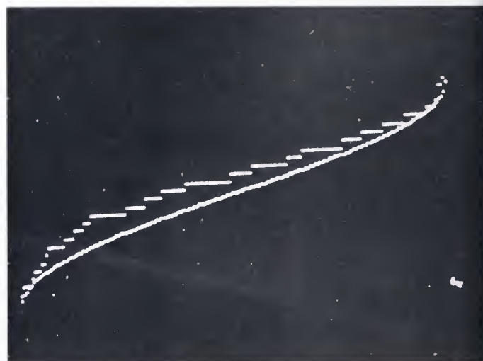
Figure 6. Co-channel beat with noise component (note noise bubble on left).
